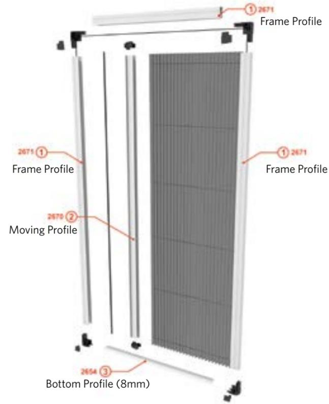
The width is 26 mm and the treshold profile's height is 8 mm.
